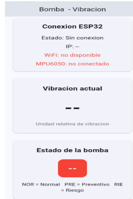
Fig. 7. Digital platform for real-time monitoring connected via Wi-Fi
