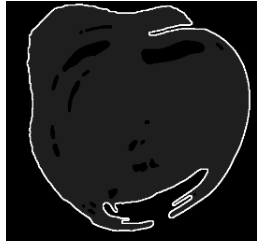
Fig. 6. Binarized frame with low blur values to appreciate droplet reflections and their contrast with the contour.
